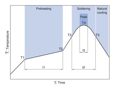
Preheating Soldering Peak Temp. Time Temp. Time Temp. Time T2 T3 **T4** t3 150°C 180°C 60 to 120s 10 to 30s 245°C 230°C 5s max.
