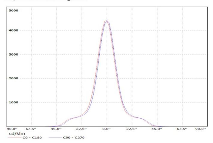
Luminaire: Ledil Oy CN12638\_LENINA-S (Cree CXA20 698Im @ 250mA) Efficiency=88% Lamps: 1 x Cree CXA20 698Im @ 250mA
