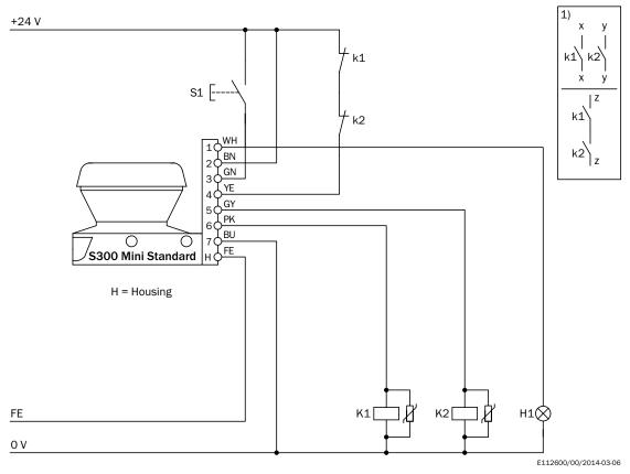
S300 Mini Standard in conjunction with relays/contactors
